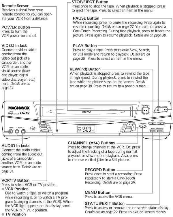
Use to watch TV (changing channels at the TV) or to watch one program while recording another. When the VCR light does not appear on the display panel, the VCR is in TV position.
